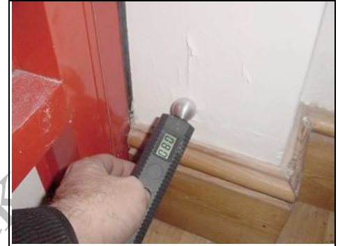
Damp front left reading 80
