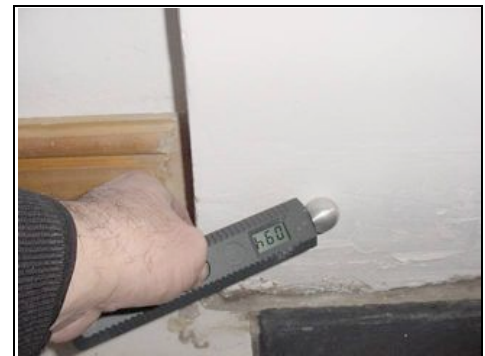
Damp middle left side reading 94
